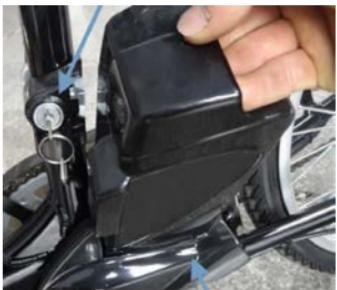
Gently push upwards so the battery fit into its housing.
